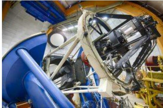
*The Dark Energy Camera is mounted on the 4-meter Blanco telescope at the Cerro Tololo Inter-American Observatory in Chile. The final day of data-taking for the Dark Energy Survey is Jan. 9. Photo: Fermilab*
