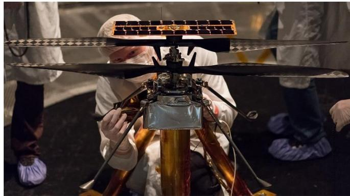
*Handling Mars Helicopter: Members of the NASA Mars Helicopter team attach a thermal film to the exterior of the flight model of the Mars Helicopter. Image Credit: NASA/JPL-Caltech.*
