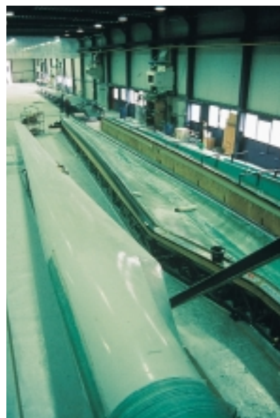
Aerpac in Scotland Aerpac designs and manufactures glass-epoxy rotor blades from 15m to 70m in diameter, for turbines of 50kW to 2MW.
