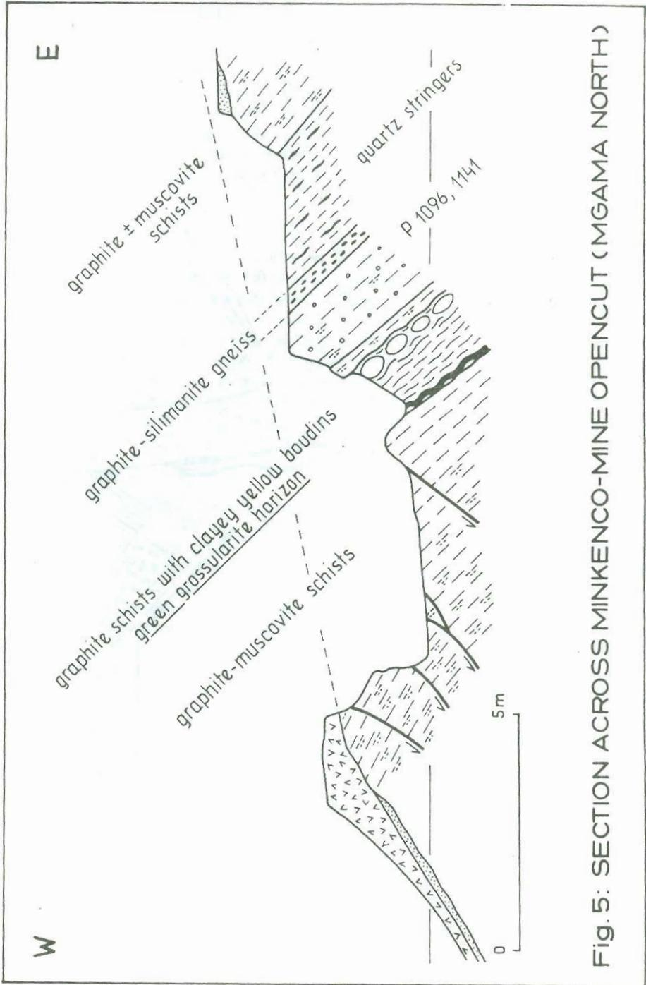
Fig. 5: SECTION ACROSS MINKENCO-MINE OPENCUT (MGAMA NORTH)
