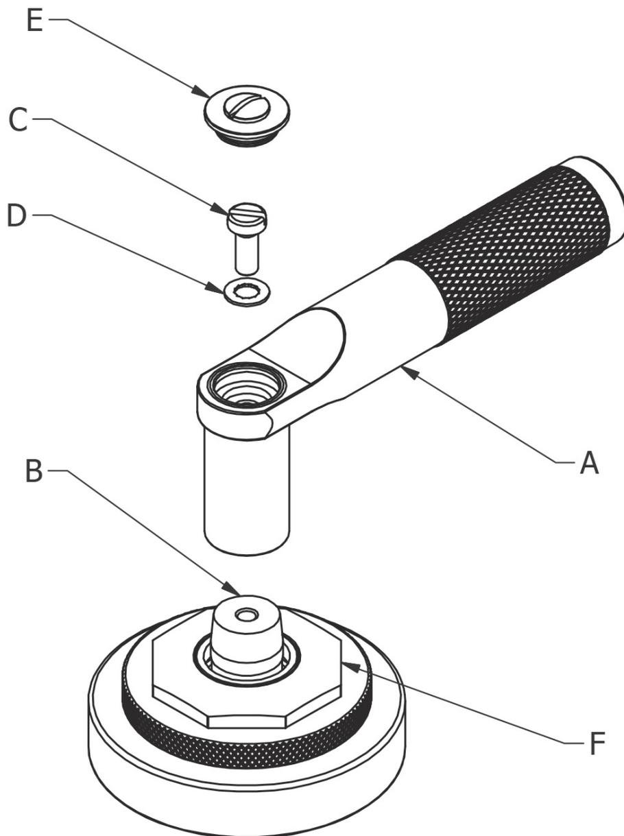
1. Screw handle (A) onto spindle (B) using screw (C) and washer (D).
