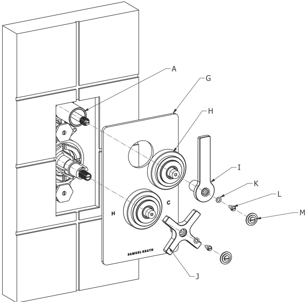
6. Apply a bead of silicon sealant to the wall where the trim plate assembly (G) will sit.
