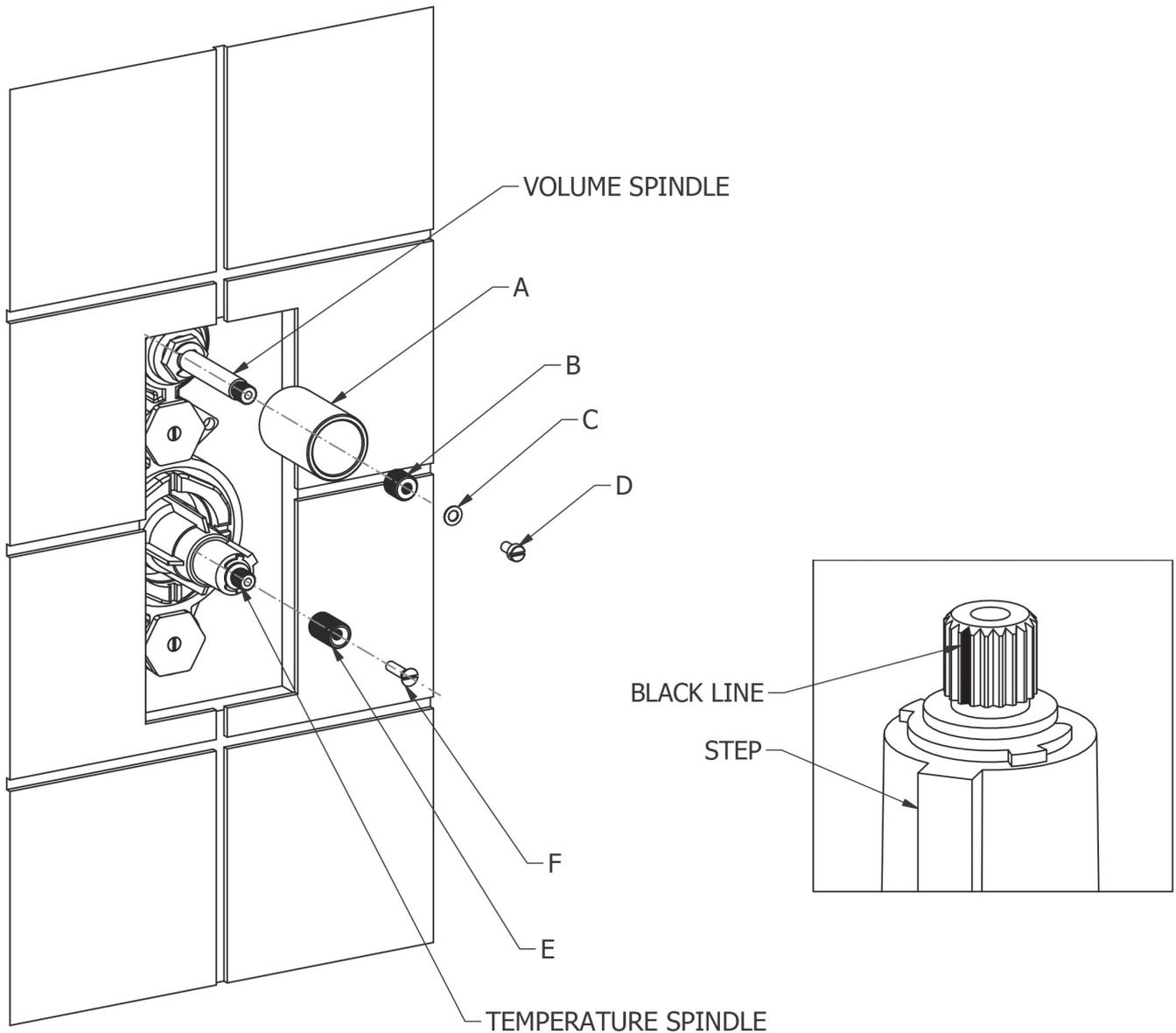
2. Ensure that the black line on the temperature spindle is in line with the step as shown
