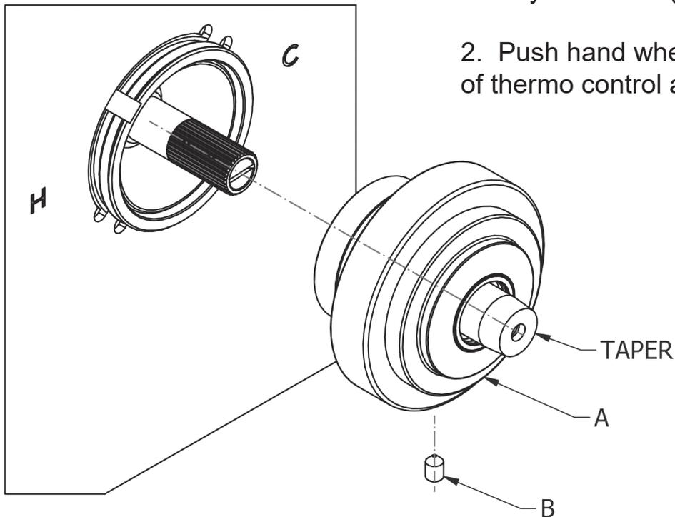
3. Using M3 screw (D), secure hand wheel (C) to thermo control assembly (A), as shown.
