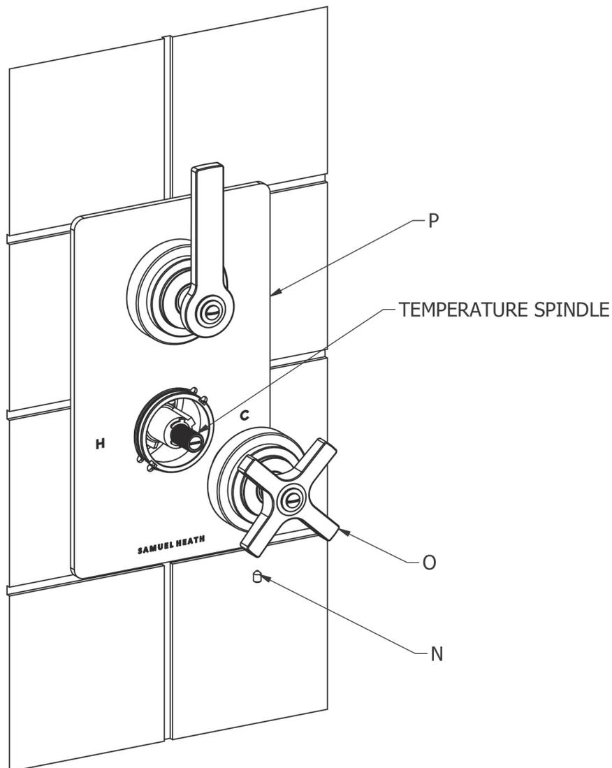
1. Remove grub screw (N) from the temperature escutcheon (O).
