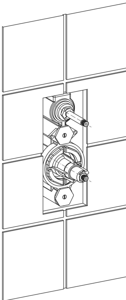
1. Install the finished surface, ensuring the finished surface is in accordance with the minimum and maximum installation depths shown on the drawings in the front of this booklet.
