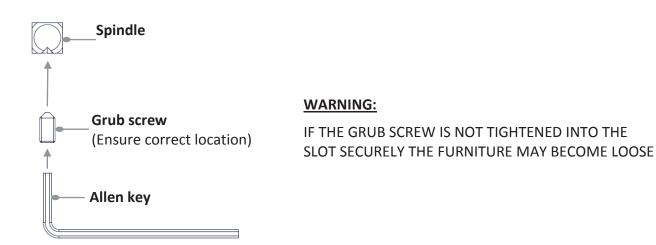
Pre Installation – We recommend the use of a strongly sprung latch for our solid door furniture, heavy sprung if using our unsprung lever handle.
