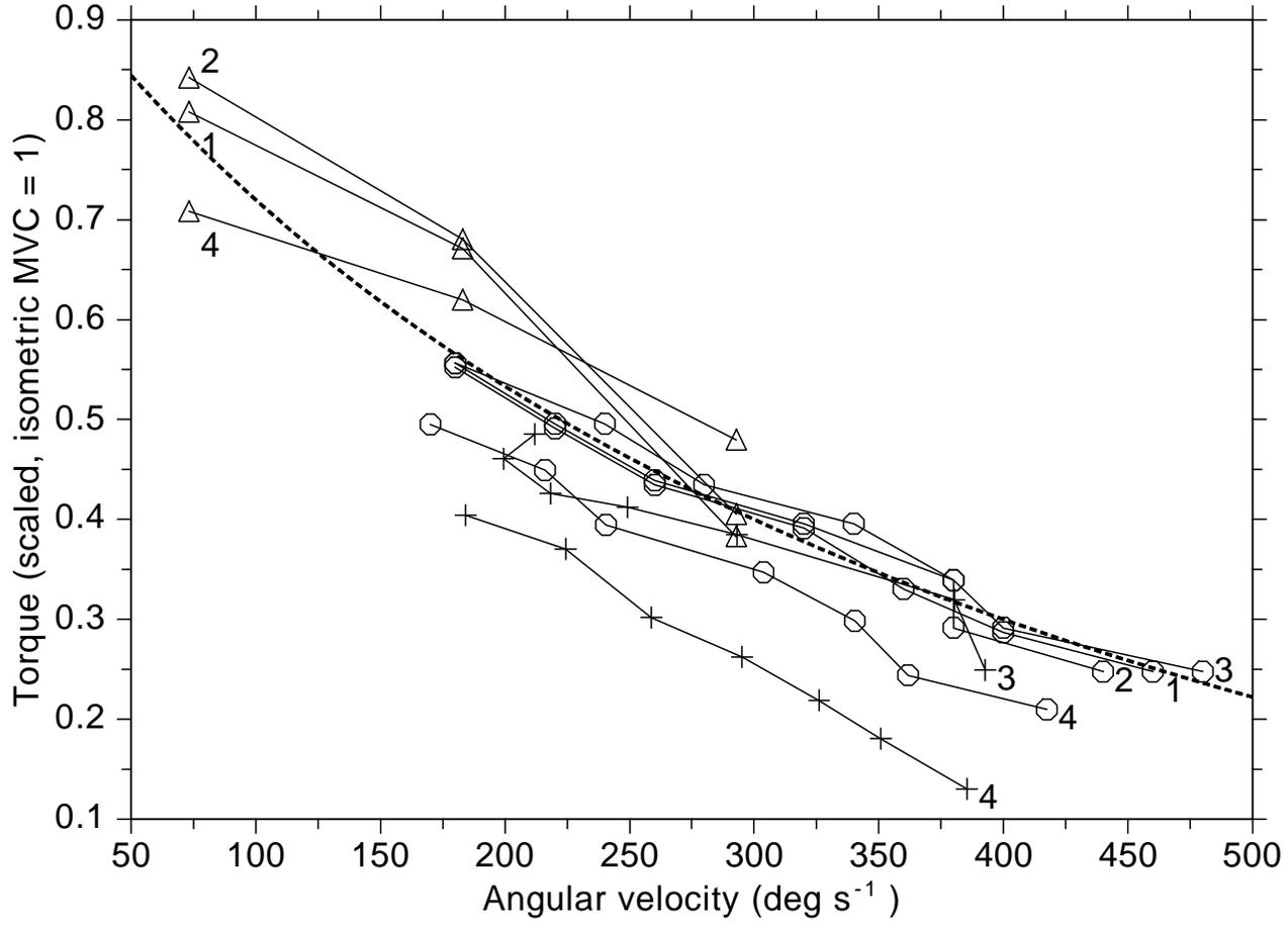
Figure 4 Torque-velocity curves for one participant determined using different calculational methods and devices.
