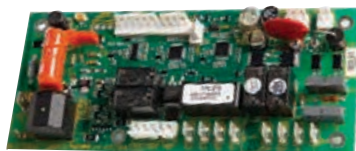
AK1264 WHALE Space/Water Heater PCB
