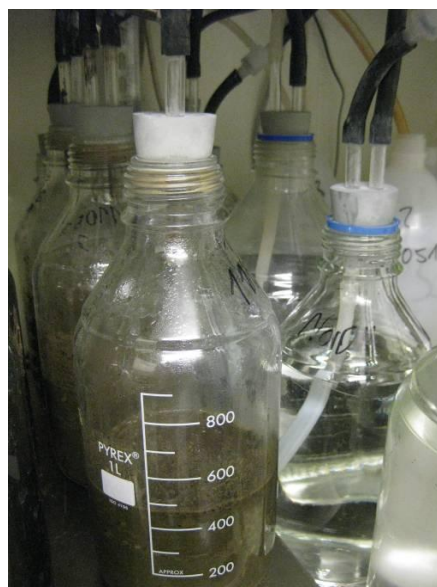
Picture 15: Analysis of biochemical methane potential or residual methane production (batch test)
