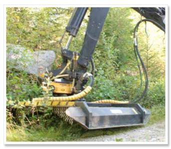
The sidewalls of our mulching heads have a sloped design. The material will fall easier to the ground while mulching. All models are equipped with a hydraulic hub motor, these motors are designed for hours of continuous operation at high-pressure. This model is fitted with a pivoting attachment, is open on the front side of the head, and has a chain curtain on the rear side. This increases safety when mulching and during forward movements.
