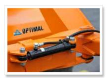
One of the booms of the integrated sideshifting system is telescopic and connected with the hydraulic lifting system. In case of impact with an obstacle, the mulching head moves backwards and upwards at the same time. After the obstacle is cleared, the head returns to the working position again.
