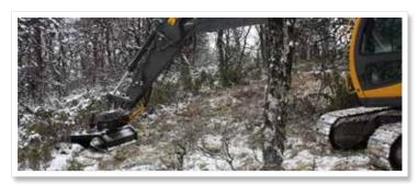
The Trejon Optimal hydraulic chain mulching heads are suitable for the work under hard conditions in hard to access terrain. For example, two type of use are for the mulching of slopes and under electric power lines.
