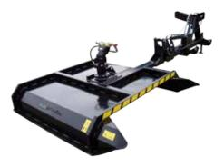
The M160H3P model with hydraulic drive. In this picture equipped is with a boom and 3pt attachment. Can also be ordered with a Volvo-BM connection.
