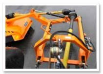
The Trejon Optimal M1650 is equipped with an integrated hydraulic sideshift. The movement pattern is 128cm wide and the mulching head has a pendular movement for proper following of the terrain. Good visibility of the entire machine is possible from the driver's seat.
