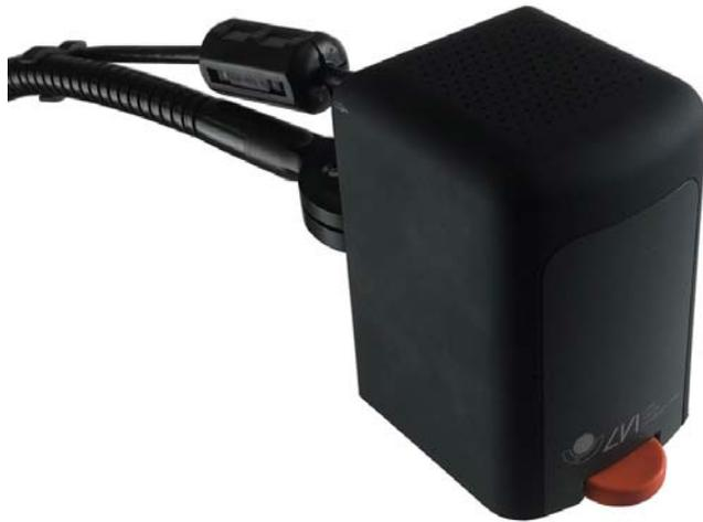
The distance camera is connected to the tablet computer using a USB cable. The camera lens can be folded down if you wish to view an object from a distance.
