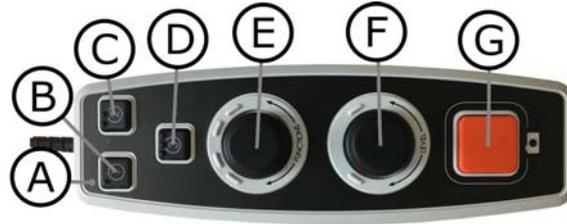
The unit can be used in simple profile or advanced profile. When the unit is in simple profile the LED lights green. When the unit is in advanced profile the LED lights blue. There is also a settings mode. When the unit is in settings mode it lights yellow.
