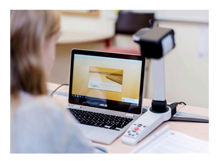
From the software you control the video magnifiers' features, such as magnification, artificial colors and brightness. The software provides you with the ability to make individual adjustments for the best possible experience!
