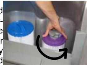
**WARNING: Power to your spa must be turned off prior to removing your filters. The suction at the filter is extremely strong and can cause injury if there is no filter. NEVER run your spa without the filters properly installed. Injury to person and damage to the equipment can occur. Any damage to equipment due to this circumstance will not be covered under warranty.**
