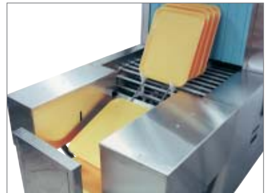
WD-40BRE. After the wash the trays are stacked on a tray dispenser.
