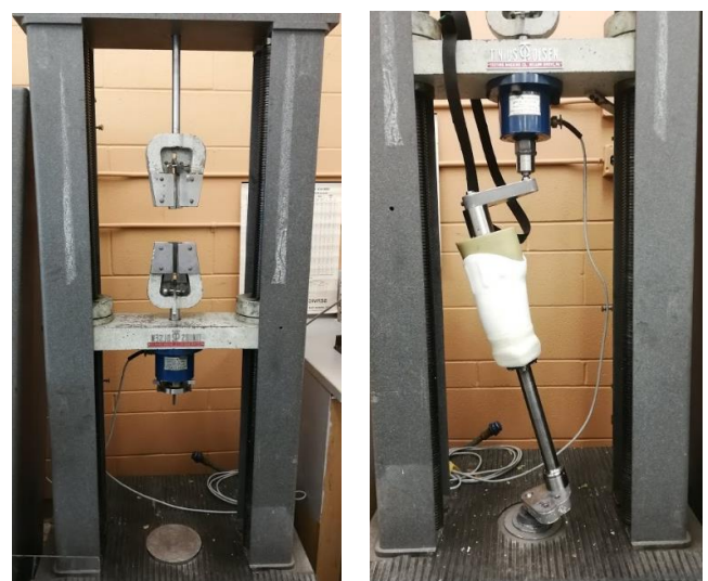
Figure 4. Left: Tinius Olsen Universal Testing Apparatus; Right: Completed set-up.
