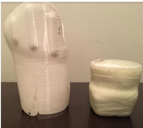
Figure 7: Complete Socket Failure
