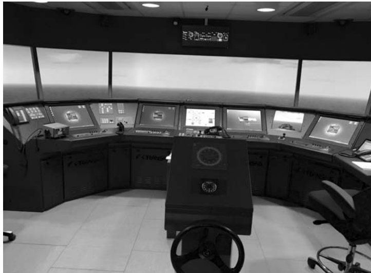
Figure 3: High-fidelity ship's bridge simulator at Chalmers University of Technology
