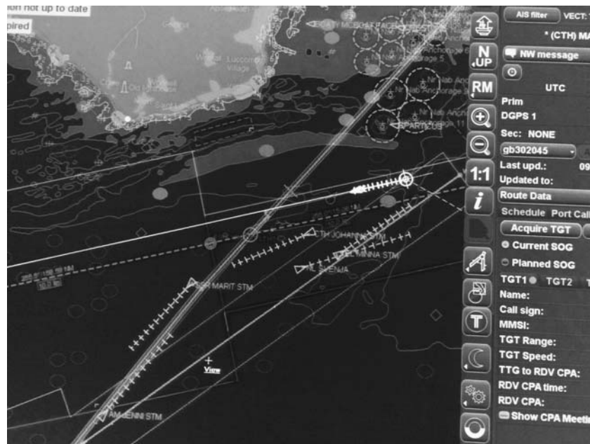
Figure 5: An ECDIS screen capture of several ships and their broadcasted routes.
