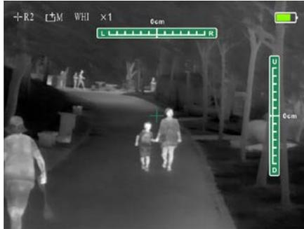
Fig 25. reticle position adjustment interface
