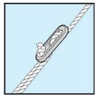
Secure each guy rope, positioning its peg at a suitable distance from the awning.
