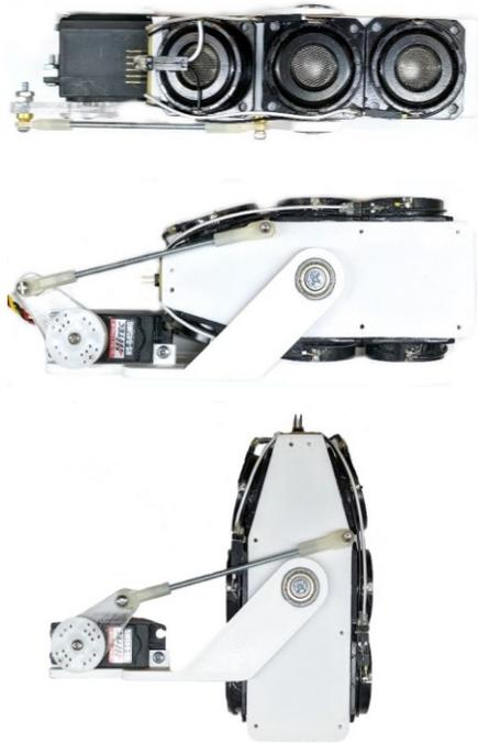
**Figure 5:** Air-vortex-ring generator with mounting assembly. The generator consists of a 3D-printed chamber, and six subwoofer transducers. The mounting assembly consists of a 3D-printed mount, to which the generator is attached at its center of mass, and a high-torque servo motor (HS-645MG) that controls the angle. The images above show the 0 degree and 90 degree angular positions of the generator relative to the screen.
