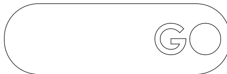
Figure A.3: Go tool used in the validating procedure (1.5 mm thickness)
