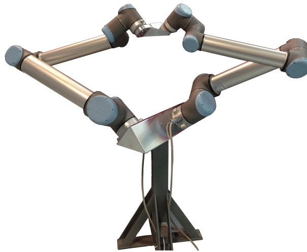
Figure 2.1: The Dual Robot Calibration method.
