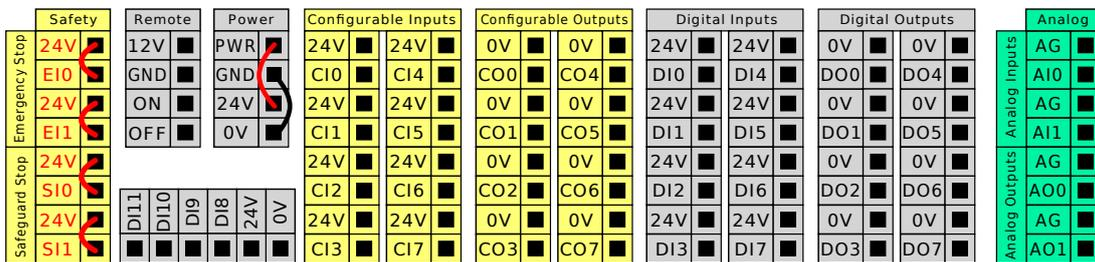
You can use the horizontal Digital Inputs block (DI8-DI11), illustrated below, for quadrature encoding conveyor tracking (see 8.3. Gemeinsame Spezifikationen für alle Digital-E/A unten) for these types of input.
