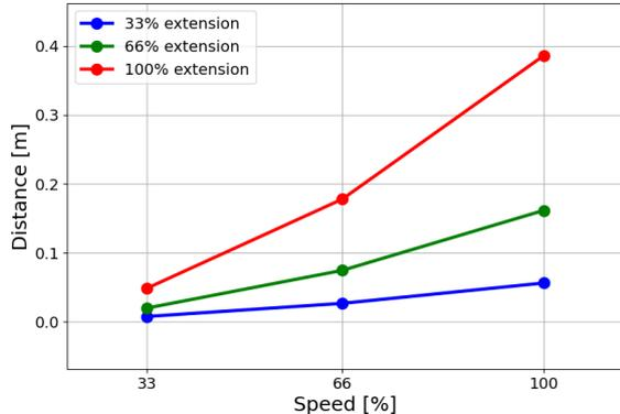
Stopping distance in meters for 66% of 20 kg:
