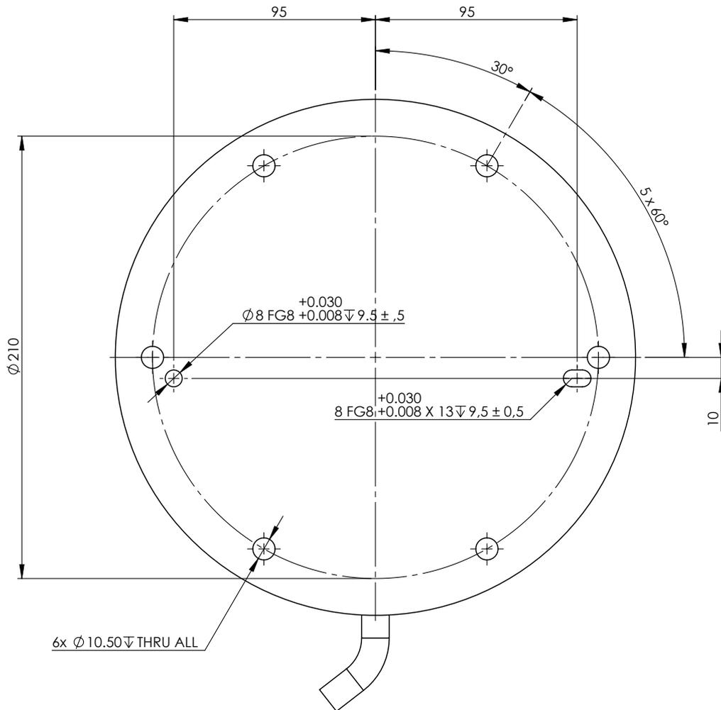
**Mounting Plate with Pins for Robot Base**
