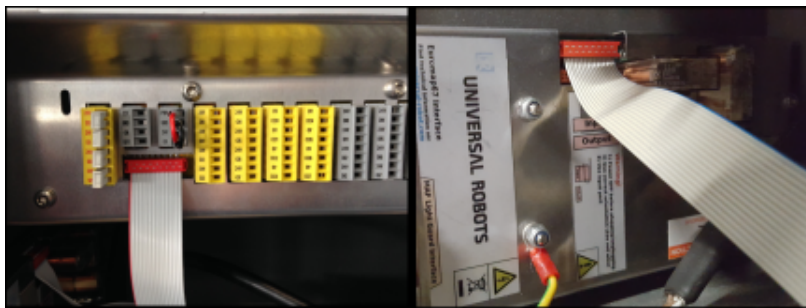
Figure 19.1: Ribbon cable connection
