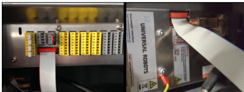
Figure 19.1: Ribbon cable connection
