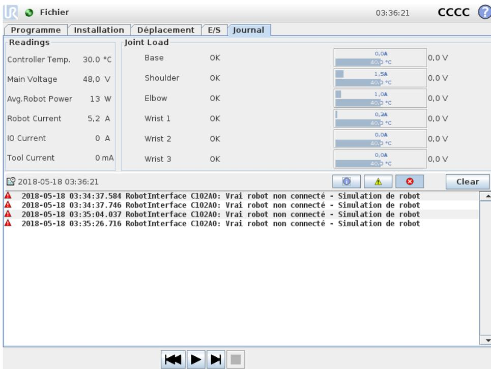
The screenshot shows the 'Journal' tab in the software interface. It is divided into two main sections: 'Readings' on the left and 'Joint Load' on the right. Below these is a log window showing error messages.
