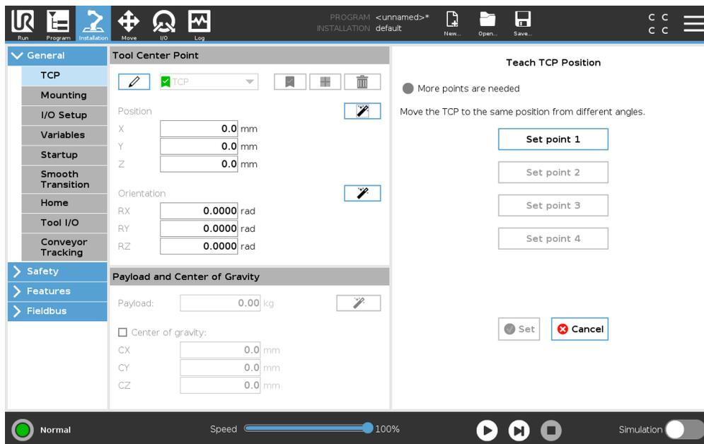
TCP position coordinates can be calculated automatically as follows:
