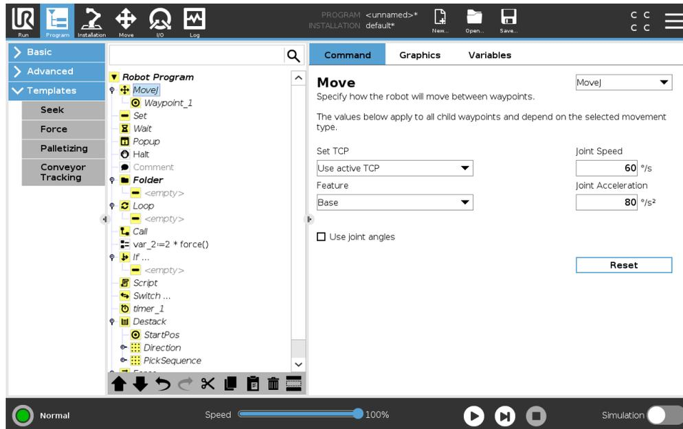
The **Move** command controls the robot motion through the underlying waypoints. Waypoints have to be under a Move command. The Move command defines the acceleration and the speed at which the robot arm will move between those waypoints.
