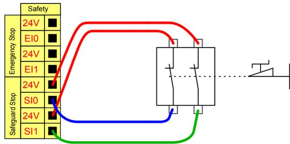
This configuration is only intended for applications where the operator cannot go through the door and close it behind him. The configurable I/O is used to setup a reset button outside the door to reactivate robot motion.
