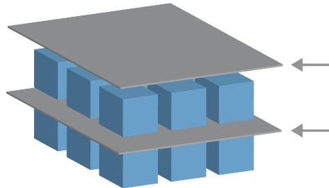
Separators, such as paper or Styrofoam, can be placed between layers in a palletizing sequence. To add separators between layers, follow the instructions below:
