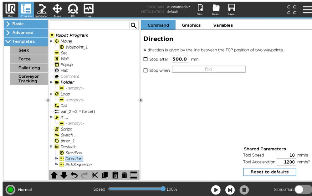
The direction is given by two positions, and is calculated as the position difference from the first positions TCP to the second positions TCP.
