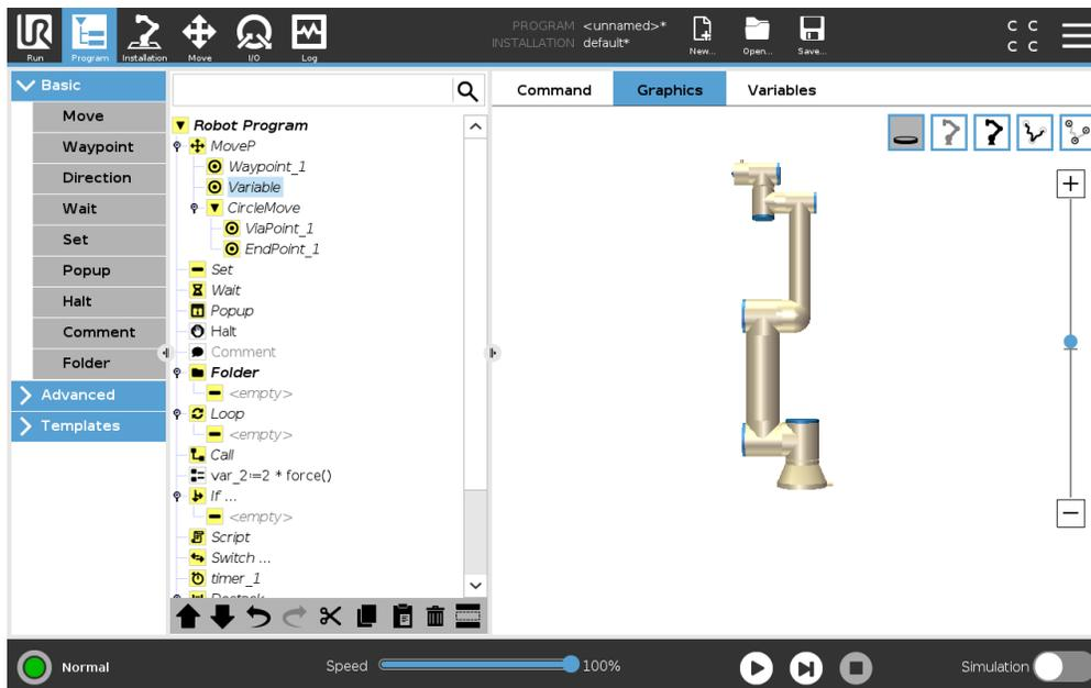
Graphical representation of the current robot program. The path of the TCP is shown in 3D view, with motion segments in black, and blend segments (transitions between motion segments) shown in green. The green dots specify the positions of the TCP at each of the waypoints in the program. The 3D drawing of the robot arm shows the current position of the robot arm, and the shadow of the
