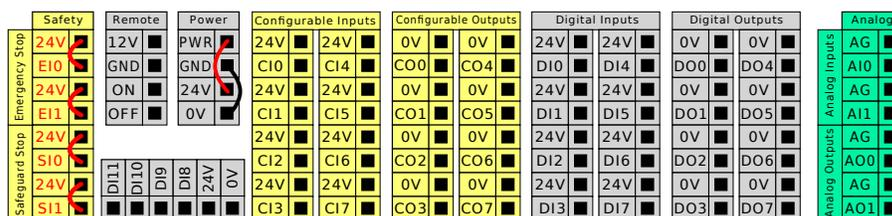
Note: You can use the horizontal Digital Inputs block (DI8-DI11), illustrated below, for quadrature encoding Conveyor Tracking (see 5.4.1) for these types of input.
