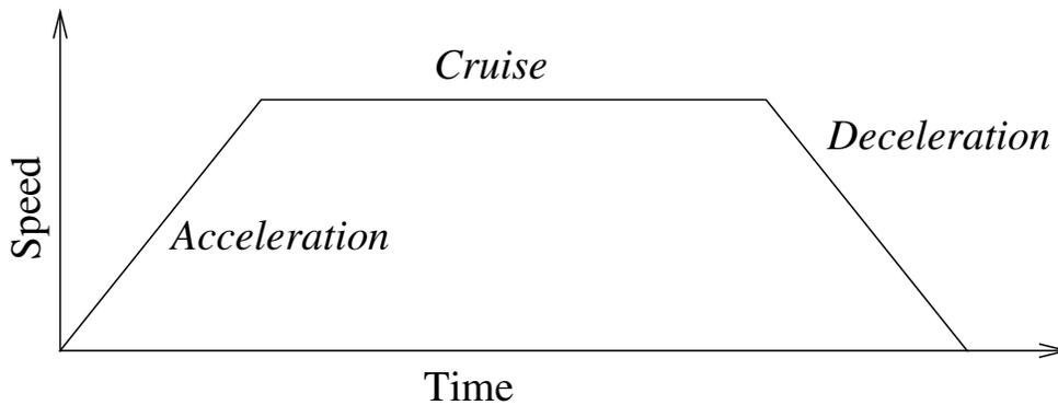
Figure 15.1: Speed profile for a motion. The curve is divided into three segments: *acceleration*, *cruise* and *deceleration*. The level of the *cruise* phase is given by the speed setting of the motion, while the steepness of the *acceleration* and *deceleration* phases is given by the acceleration parameter.
