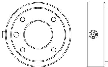
This connector provides power and control signals for grippers and sensors used on a specific robot tool. The industrial cable listed below is suitable:
