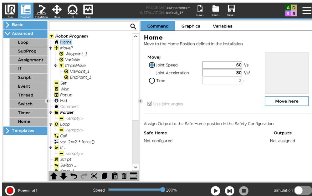
The Home node uses joint angles to move the robot to a predefined Home position. If defined as a Safe Home position, the Home node displays as Home(Safety) in the Program Tree. If the Home
