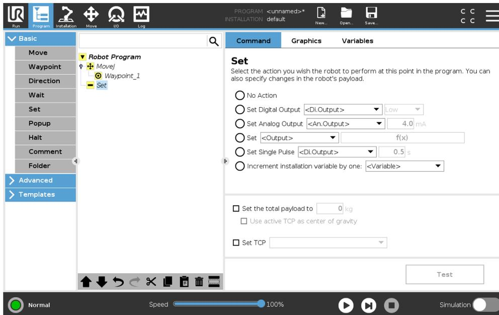
Sets either digital or analog outputs to a given value. Digital outputs can also be set to send a single pulse.
