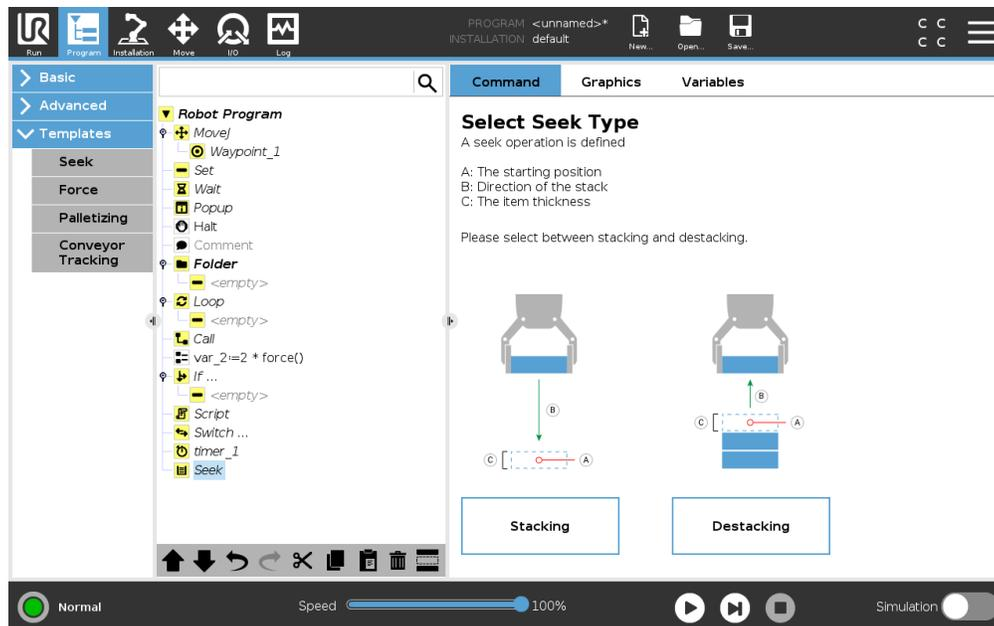
When stacking, the robot arm moves to the starting position, and then moves *opposite* the direction to search for the next stack position. When found, the robot remembers the position and performs the special sequence. The next time round, the robot starts the search from the remembered position incremented by the item thickness along the direction. The stacking is finished when the stack
