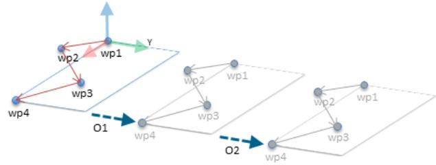
Figure 16.6: Applying an offset to the plane feature
