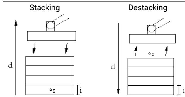
When programming a seek operation for working on a stack, one must define  $s$  the starting point,  $d$  the stack direction and  $i$  the thickness of the items in the stack.
