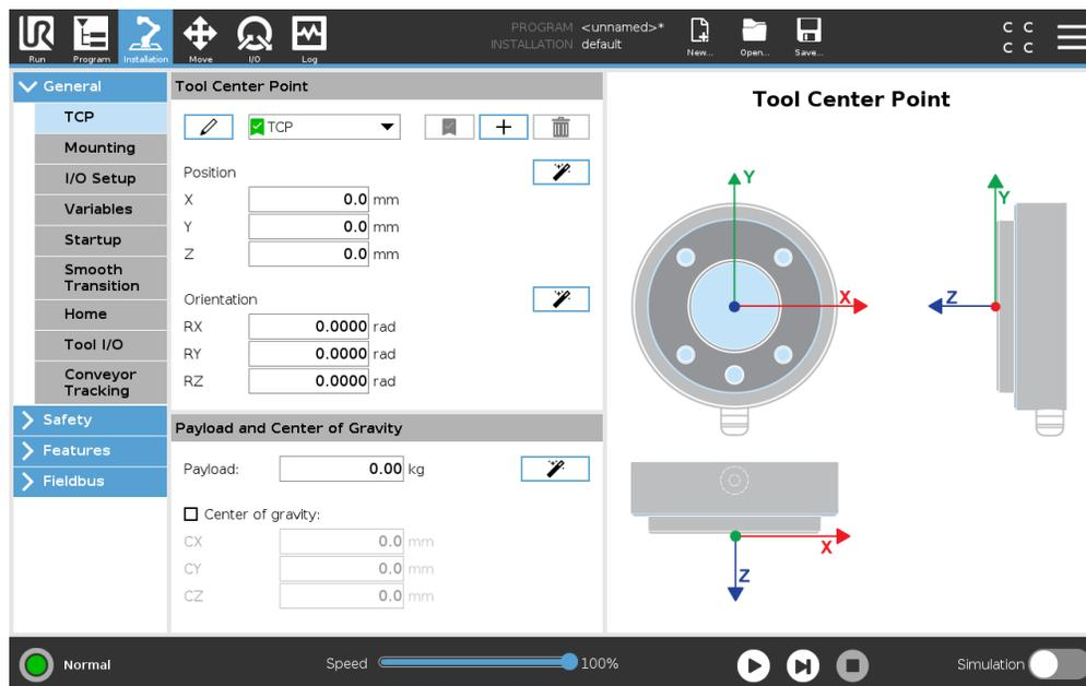
A **Tool Center Point** (TCP) is a point on the robot's tool. The TCP is defined and named in the Installation Tab **Setup for the Tool Center Point** screen (shown above). Each TCP contains a translation and a rotation relative to the center of the tool output flange.
