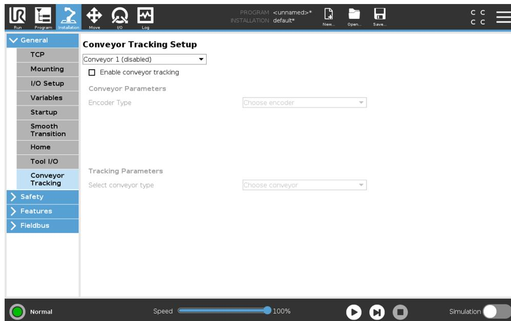
The Conveyor Tracking program node is available in the Program Tab under Templates. All movements under this node are allowed while tracking the conveyor, but they are relative to the motion of the conveyor belt. Blends are not allowed when exiting Conveyor Tracking, so the robot stops completely before making the next motion.
