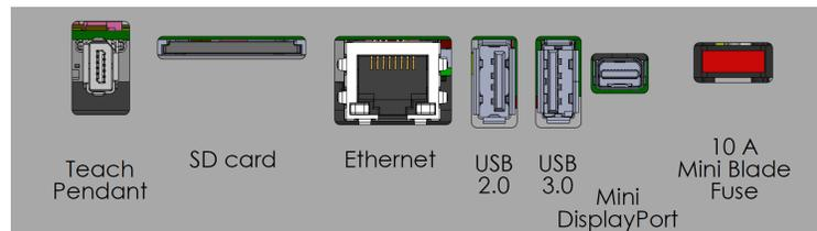
Note: The Fuse must be UL marked, Mini Blade type with maximum current rating: 10A and minimum voltage rating: 32V
