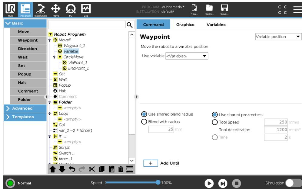
A waypoint with the position given by a variable, in this case `calculated_pos`. The variable has to be a *pose* such as
