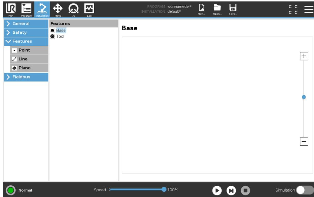
The **Feature**, is a representation of an object that is defined with a name for future reference and a six dimensional pose (position and orientation) relative to the robot base.
