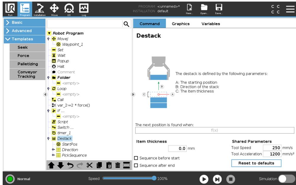
When destacking, the robot arm moves from the starting position in the given direction to search for the next item. The condition on the screen determines when the next item is reached. When the condition becomes satisfied, the robot remembers the position and performs the special sequence. The next time round, the robot starts the search from the remembered position, incremented by the item thickness along the direction.
