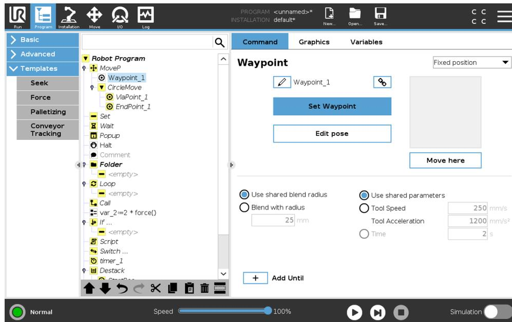
A point on the robot path. Waypoints are the most central part of a robot program, telling the robot arm where to be. A fixed position waypoint is taught by physically moving the robot arm to the position.
