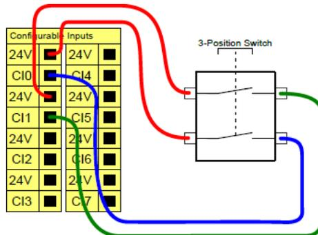
Note: The two input channels for the Three-Position Enabling Device input have a disagreement tolerance of one second.
