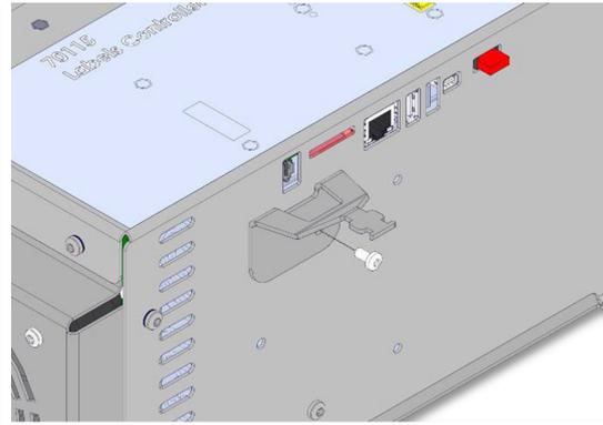
6. Serrez la vis incluse (Couple 1 Nm)
