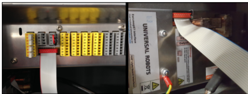
Figure 19.1: Ribbon cable connection
