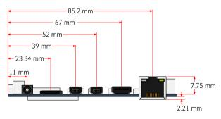
Figure 2: Mounting holes and dimensions of the VAB-600
