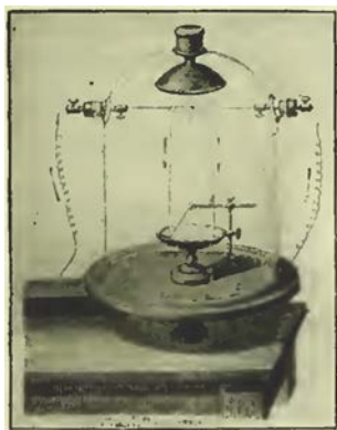
FIG. 3. TRANSMISSION OF HEAT THROUGH A VACUUM.
