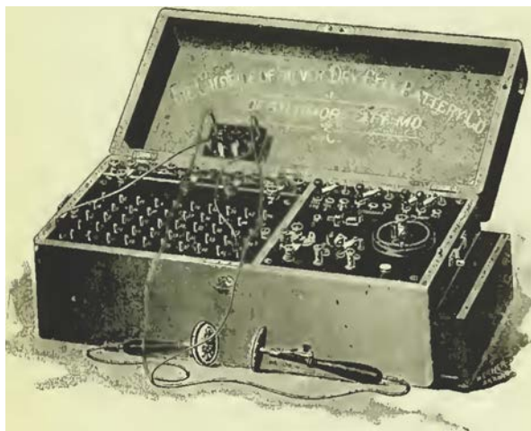
FIG. 103.- INDUCTION COIL WITH BATTERY OF CHLORIDE OF SILVER CELLS.
