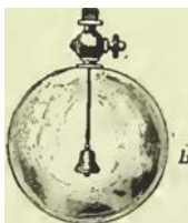
FIG. 2.-TRANSMISSION OF SOUND THROUGH A VACUUM.
