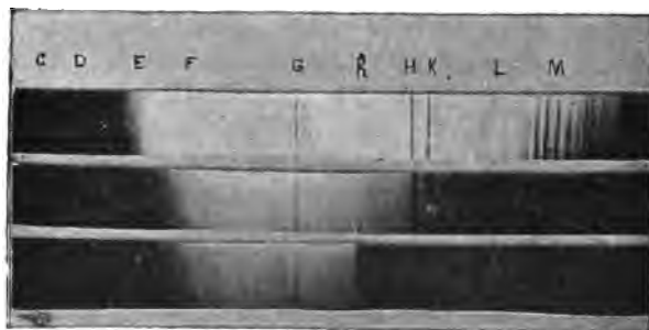
FIG. 43.— Photographs showing the disappearance of the solar ultra-violet on certain days caused by unknown influences. —The upper band represents an ordinary solar spectrum extending to the borders of the N ray. The band beneath it shows the disappearance of the solar ultra-violet starting from the L ray, notwithstanding the prolongation of the exposure. The lower band represents the total disappearance of the ultra-violet when the spectrum is photographed through a transparent solution of sulphate of quinine.
