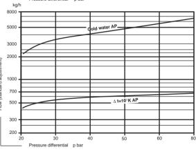
In the presence of cold water the bimetallic strips remain flat. As the temperature increases the discs change shape, becoming convex, and displacing the plug against the seating. The maximum convexity, which coincides with a fully tight shut off is obtained just at the point when the condensate turns to steam.
