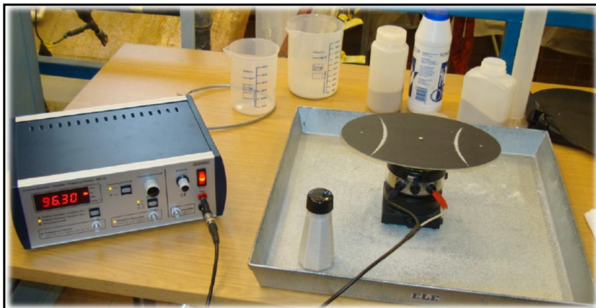
Figure 4 : Experimental Apparatus for Chladni Plate investigation.
