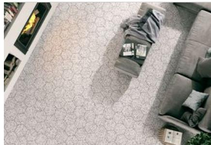
**DONNÉES TECHNIQUES****NOM:** Hex 25 Venice White RD3**CODE:** PT05291**SÉRIE:** Venice Hex 25**FORMAT:** 22x25 Hexagonal**TYPE DE PIÈCES:** BASE**TYPE DE SUPPORT:** Grès Cérame**ASPECT:** Stone**FINITION:** Mate**USAGE:** Sol et Mur**DESTONATION:** V2 Léger**GLISSEMENT - NORME UNE:** Clase 3**% ABSORPTION:** E < 0.5%**RÉSISTANT AU GEL:** OUI**NOMBRE DE VISAGES:** 21
