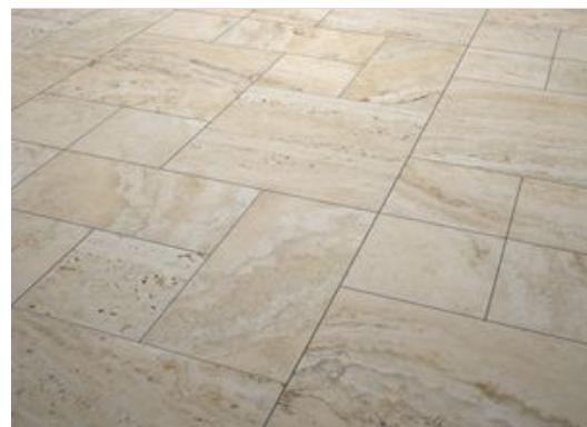
**DONNÉES TECHNIQUES****NOM:** Siena Beige Modular**CODE:** PT04152**SÉRIE:** Siena**FORMAT:** 50x50 Modular**TYPE DE PIÈCES:** BASE**TYPE DE SUPPORT:** Grès Cérame**ASPECT:** Modular**FINITION:** Satiné**USAGE:** Sol**DESTONATION:** V4 Considérable**GLISSEMENT - NORME UNE:** Clase 2**% ABSORPTION:** E < 0.5%**RÉSISTANT AU GEL:** OUI**PEI:** 4
