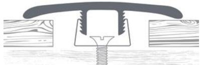
**TECHNICAL DATA****CODE:** QUTM-SS-TM**NAME:** T-Mold 4562-Seashell**SERIES:** Timber Ridge Platinum 20**FINISH:** Natural**LOOK:** Wood Look**SUITABLE FOR:** Indoor**TYPOLOGY:** SPC Flooring**TYPE OF PIECE:** Transition molding**USE:** Floor only**FAMILY:** Waterproof Wall and Floor Covering**NOTES:** This Product Is An Spc/Waterproof Material And Not A Ceramic Tile.
