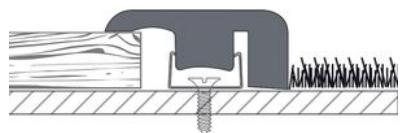
**TECHNICAL DATA****CODE:** QUTM-NU-EC**NAME:** End Cap 2004-Nutmeg Oak**SERIES:** Timber Ridge Platinum 20**FINISH:** Natural**LOOK:** Wood Look**SUITABLE FOR:** Indoor**TYPOLOGY:** SPC Flooring**TYPE OF PIECE:** Transition molding**USE:** Floor only**FAMILY:** Waterproof Wall and Floor Covering**NOTES:** This Product Is An Spc/Waterproof Material And Not A Ceramic Tile.
